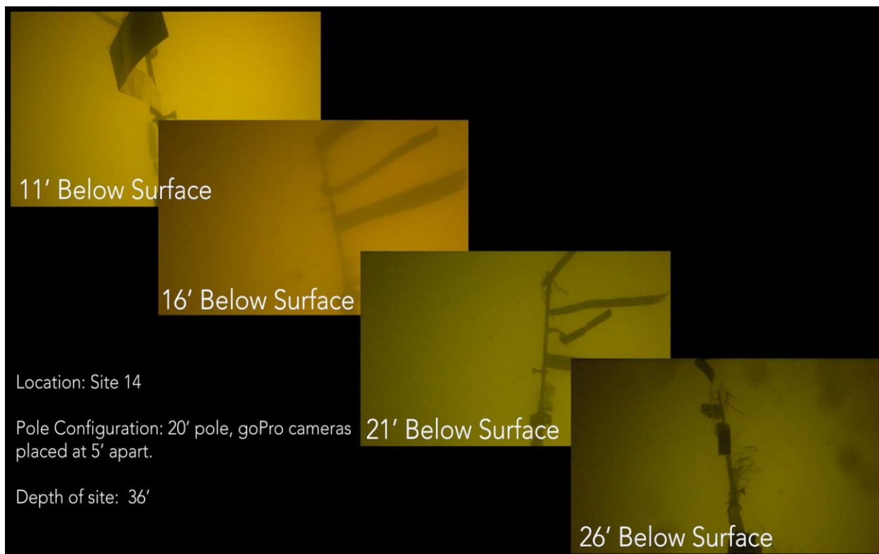
Figure 10 Propeller Downwash Impacts of at least 26 feet Depth by Wake Board Boat in Surf Mode. (Test Site 14) Lake Waramaug, 2024
